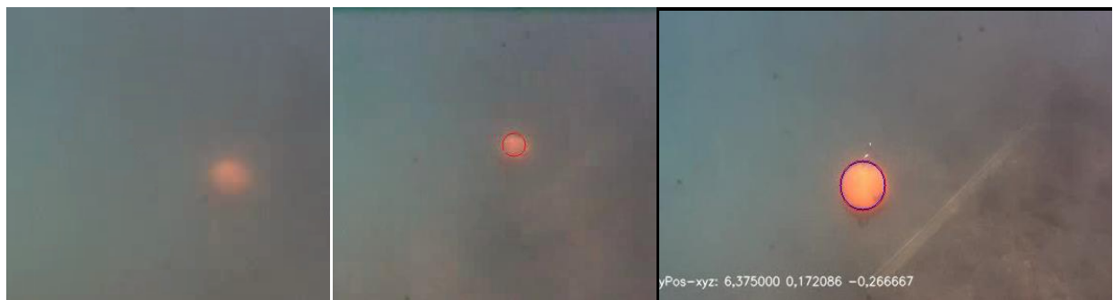
Figure 4b: SAUC-E 2011 Bremen's buoy servoing: detection, initial lock on it, final tracking and circling around it. This will be an anomaly for Task 3 in SAUC-E'13.
